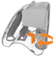
Hold the dirty water tank over a sink and pull to open the quick pour spout.
