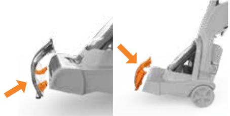
To replace the nozzle, line up the tabs on the nozzle with the tabs underneath the front of the carpet washer. Push the nozzle down until it clicks into place.
