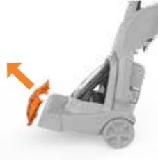
Remove both tanks and tilt the carpet washer back. Lift the nozzle from the top and pull forward to remove.
