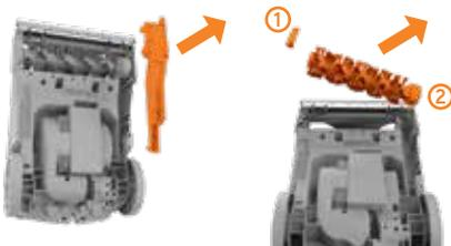
Pull to remove the belt cover. Lift the brushbar out from the left hand side first and unloop the brushbar from the belt. Pull the brushbar to remove from the carpet washer.
