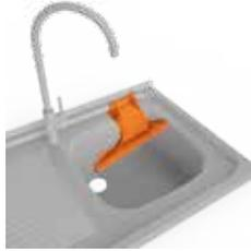
Rinse the nozzle under water to remove dirt/debris.
