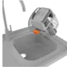
Empty the dirty water over the sink. Rinse the dirty water tank under water (max 40°C) to remove dirt/debris.
