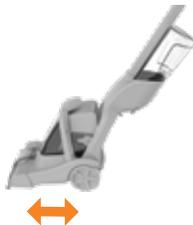
For best results apply water/solution on the forward stroke and release the trigger on the backward stroke to pick up water/solution. For a dryer finish, follow with an additional dry stroke with no trigger pressed.
