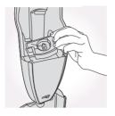
Lift to remove the hard water filter.
