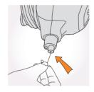
After floor head is removed, using a thin object such as a paper-clip (in the area shown), insert to remove the blockage.\*
