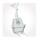
Pour 50ml of Vax detergent and 250ml of water into the detergent tank then replace cap and twist clockwise to tighten.
