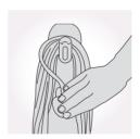
Wrap the power cord around the quick cord release hooks.
