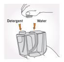
Twist water cap anti-clockwise and lift to remove.
