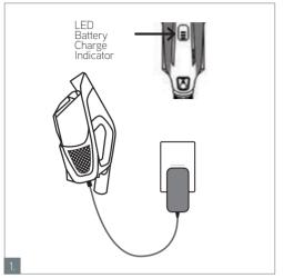
Plug in and charge the unit until all three lights are off. Charge fully for best performance. (May take up to three hours)
