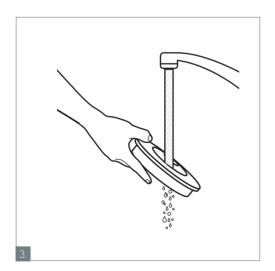
Rinse filter with water until the dirt is no longer coming out from filter. Shake it out and then let it dry for 24 hours or until completely dry.
