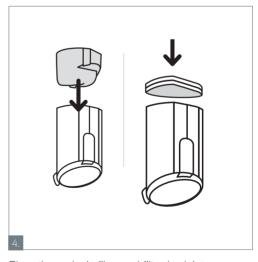
Place the cyclonic filter and filter back into the dirt cup.
