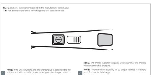
Plug in charger. Power must be off in order to recharge.
