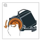
Post motor filter is located in the right side wheel. Hold the centre of the wheel and twist wheel cover anti-clockwise.
