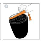
Lift out the pre-motor filter.
