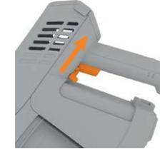
For continuous power squeeze the trigger and push the 'Continuous power latch' towards the trigger. This will lock it into the 'On' position and will continue to power the machine without having to hold in the trigger. Release the trigger to switch the machine 'Off'. Push the latch away from the trigger to unlock and release the trigger.
