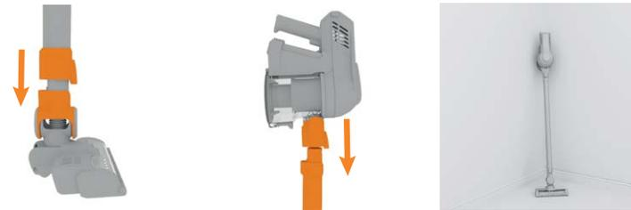
Line up the connector on the reach wand with the Powered Head. Push the reach wand down onto the Powered Head until it clicks into place.
