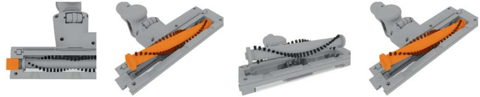
Slide to release the brushbar. The cover can not be removed.
