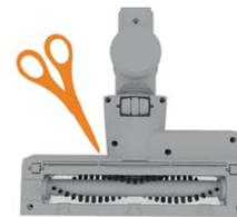
The brushbar should be removed from the Powered Head before attempting to remove any blockages. Using scissors, carefully remove any threads or hair from around the brushbar and clear any dirt or debris from Powered Head.
