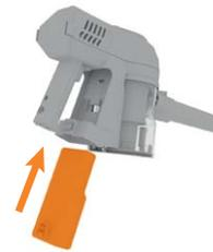
Slide the battery into the back of the handheld. The battery will click into position when correctly fitted.
