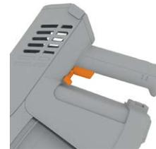
For continuous power squeeze the trigger and push the 'Continuous power latch' towards the trigger. This will lock it into the 'On' position and will continue to power the machine without having to hold in the trigger. Push the latch away from the trigger to unlock and release the trigger.
