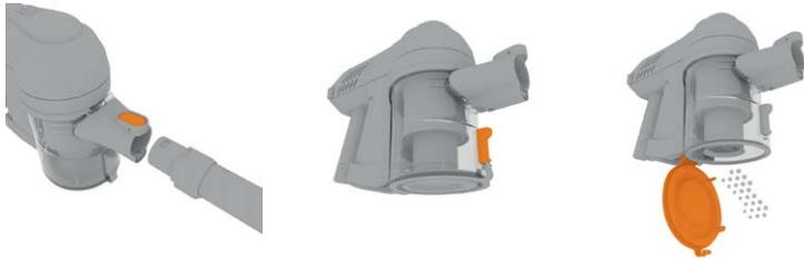
Press the handheld release clip. Pull to separate the handheld from the reach wand.
