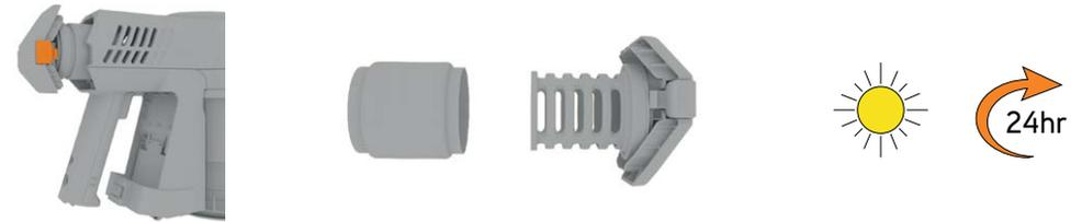
Press the filter cover release buttons located on both sides of the filter cover and pull to remove the filter from the machine.
