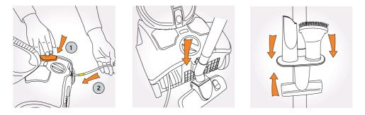
**NOTE:** For convenience there is a parking slot located at the rear of the vacuum cleaner where the floor head and tubes can be attached for storage and carrying.
