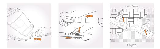
**NOTE:** The Turbobrush, hard floor tool, crevice tool, upholstery tool and dusting brush can all be attached directly to the telescopic tube or hose handle.
