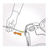
Fully unwind the power cord. A yellow mark on the cord indicates the recommended cord length. Do not exceed the cord length beyond the yellow mark.
