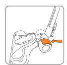
To suck up excess water push the rocker switch to the front.
