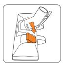
To put down water, push the rocker switch towards the back of the hard floor wash head.
