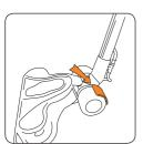
To put down water and solution and turn the brushes on, push rocker switch towards the back of the floor head.
