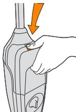
Press the twin tank release button and lift the twin tank by the handle
