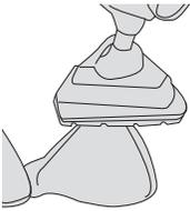
Place the microfibre pad on the floor white side facing up. Place steam mop onto pad making sure the entire pad covers the floor head
