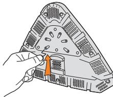
Remove cleaning pad and inspect steam mop base for blockages. If a blockage can be seen use a small thin object such as a paper-clip insert to remove
