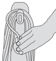
Wrap the power cord around the quick cord release hooks
