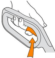
To produce steam, squeeze the trigger. To prevent over wetting floors avoid holding the trigger continuously
