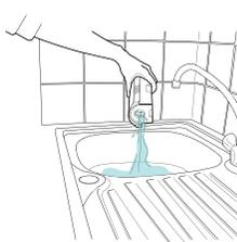
Empty any excess water, replace water cap and turn clockwise to tighten
