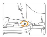
Secure the handle in place with one of the screws provided.
