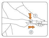
To remove/release tubes, press latch as shown.
