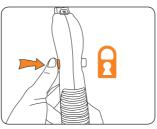
Ensure steam handle safety latch is on before heating.
