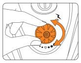
Rotate variable steam dial to adjust pressure.
