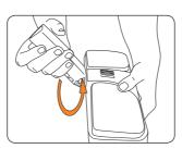
Rotate floor head connector into place.
