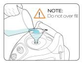
Slowly pour liquid into water tank. NOTE: Maximum tank capacity is 1.6L (2.2 jugs)
