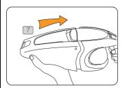
Allign bottom of the dirt container first and clip nozzle on.
