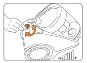
**NOTE:** Fully unwind the power cord. A yellow mark on the cord indicates the recommended cord length. Do not exceed the cord length beyond the yellow mark.
