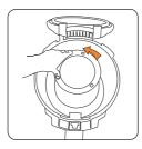
The pre-motor filter is found in the centre of the dirt container. Rotate the filter retaining disc anti-clockwise to gain access to the filter.
