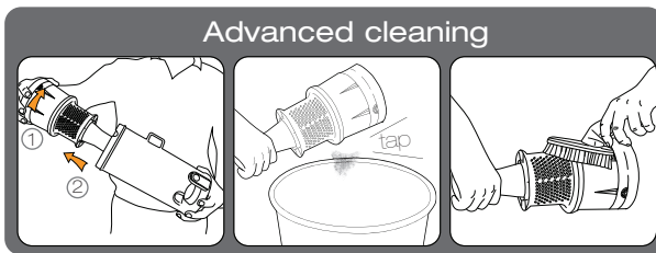
Slide out the cyclone separator. Tap over a bin to remove excess dirt or use a brush to gently clean separator.
