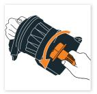
Hold the container and turn the cyclone separator anti-clockwise.
