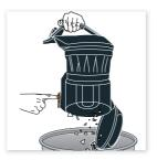
Hold dirt container over a bin and press dirt release button to open, allowing dirt to fall out.
