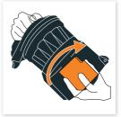
To remove the inner shroud, hold the container and rotate the shroud clockwise.
